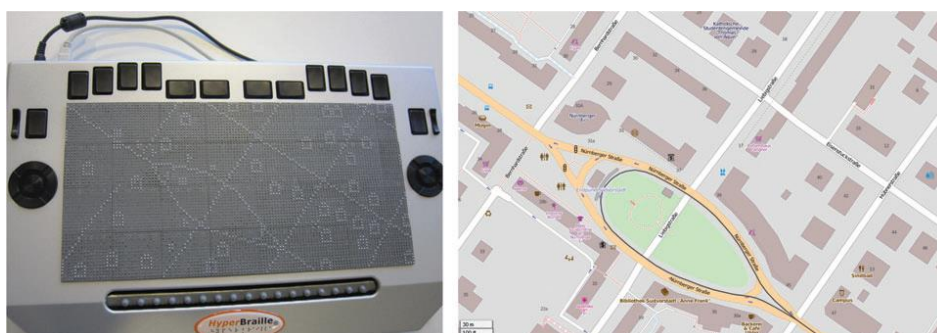
Figure 2.21. The BrailleDis 9000 tablet, composed of 7200 pins, was used in [348] to give visually impaired users access to dynamic maps. Retrieved from [348].
