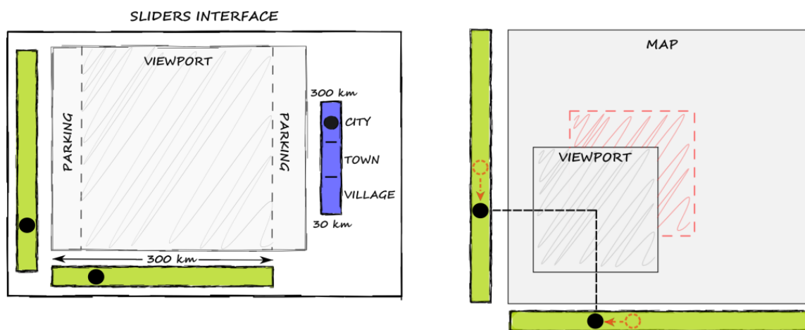
Figure 5.4. Description of the Sliders interface. Left: for panning, users can move the viewport horizontally and vertically by moving two robots (black dots on the green areas) that represent the position of the viewport's center. Users can move the third robot in the zooming area (blue area) to select any scale between 30 km and 300 km. Right: illustration of two successive sliders' and the viewport's positions over the map.
